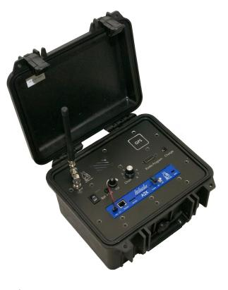
The A2FX will decode ALERT2 messages regardless of modulation polarity, and supports the Configurable FEC, for faster data rates, and encryption extensions, for secure communications, to the ALERT2 protocol. A switch on the A2FX allows the selection of one of eight radio channels, which provides coverage across a wide range of frequencies.
